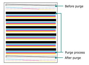
If this process does not improve the print quality, your print cartridges may be low in ink. Replace the print cartridge, if necessary.
